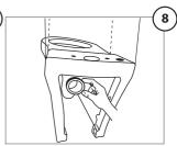
· Apply suitable lubricant around waste outlet before connecting to the bend.
