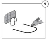
· Apply industrial paste along inside of peripheral outline on floor.
