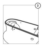
Measure thickness of water closet foot near fixing-hole area (t)
